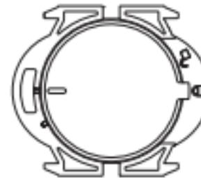
2. Place a new battery into the battery holder. Align the position mark to the opening position and press down the battery cover. After pressing the whole cover into the battery holder, rotate the position mark clockwise to the locking position.
