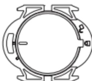
2. Place a new battery into the battery holder. Align the position mark to the opening position and press down the battery cover. After pressing the whole cover into the battery holder, rotate the position mark clockwise to the locking position.
