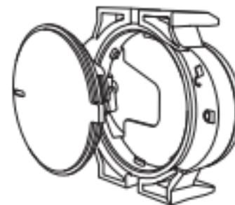
1. Rotate the position mark on the battery cover anticlockwise from the locking position to the opening position. Then open the battery holder.
